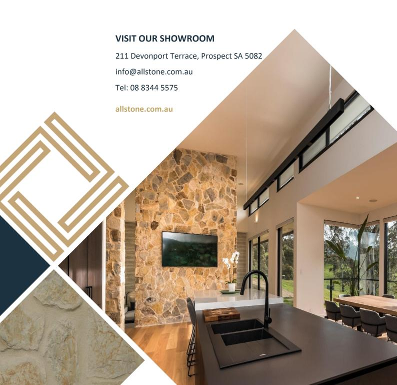
Natural stone veneers are thin pieces of stone (typically between 10 - 35mm thick) that are fixed to walls or floors (the 'substrate') with an appropriate adhesive.
